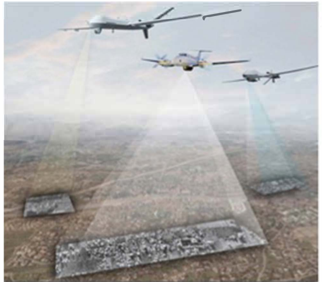
Synthetic Aperture Radar with Ground Moving Target Indicator
